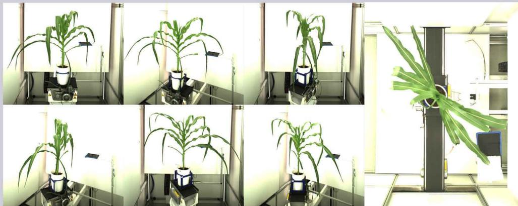
The camera input from the PHENOVISION system comprises 180° views and a top view of the object maize plant. Because of the enormous volume of data, we require a fast and accurate 3D reconstruction technique. Voxel carving fits well, but requires segmented input images.
