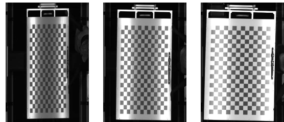
Fig. 2. The double nature of the camera model becomes apparent when imaging a checkerboard at different heights: note that the imaged width of the board depends on the distance to the camera, but the imaged length is invariant.
